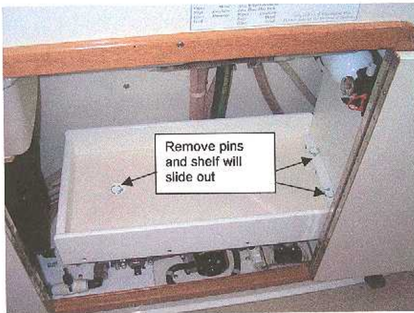
Figure 2.8 Potable water system – equipment mounted in the cabinet under the galley sink (photo taken from aft cabin looking forward – cabinet doors and horizontal shelf removed for picture)
